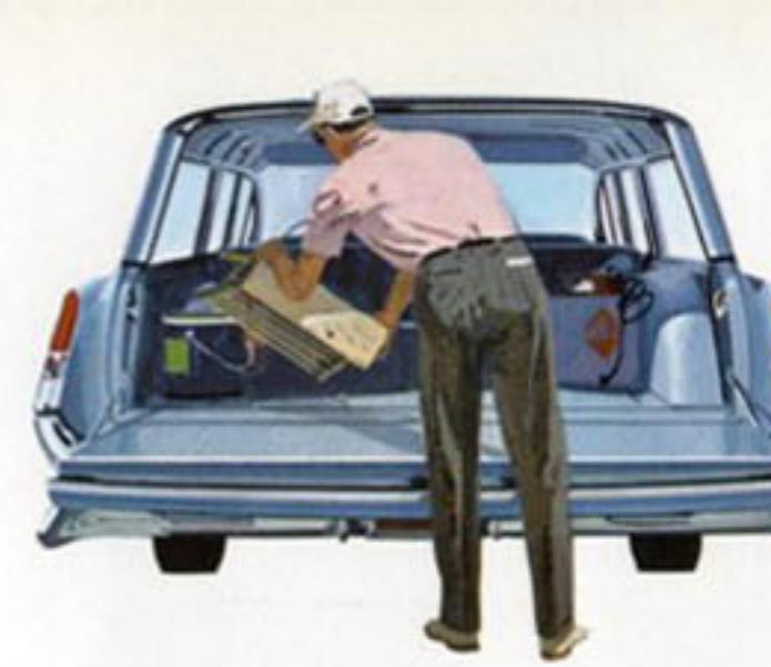
Second seat folds into floor to accommodate over 85 cu. ft. of family cargo! Below-deck Luggage Locker, optional at extra cost, lets you lock additional gear out of sight . . . holds 8 cubic feet!
