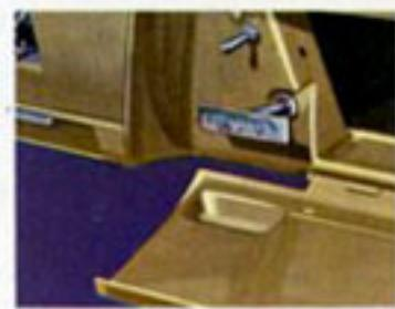
**DECK LID POWER LOCK RELEASE** opens trunk automatically from control in glove compartment.
