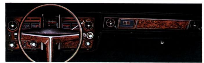
Toronado's new instrument panel is rich with inlays and gleaming with purpose. Switch and control identifications are now back-lighted for easier nighttime use; a new pushbutton ashtray is relocated for greater convenience; and the glove compartment has greater capacity. Note the distinctive drum-type speedometer, which permits you to determine your speed at a glance.
