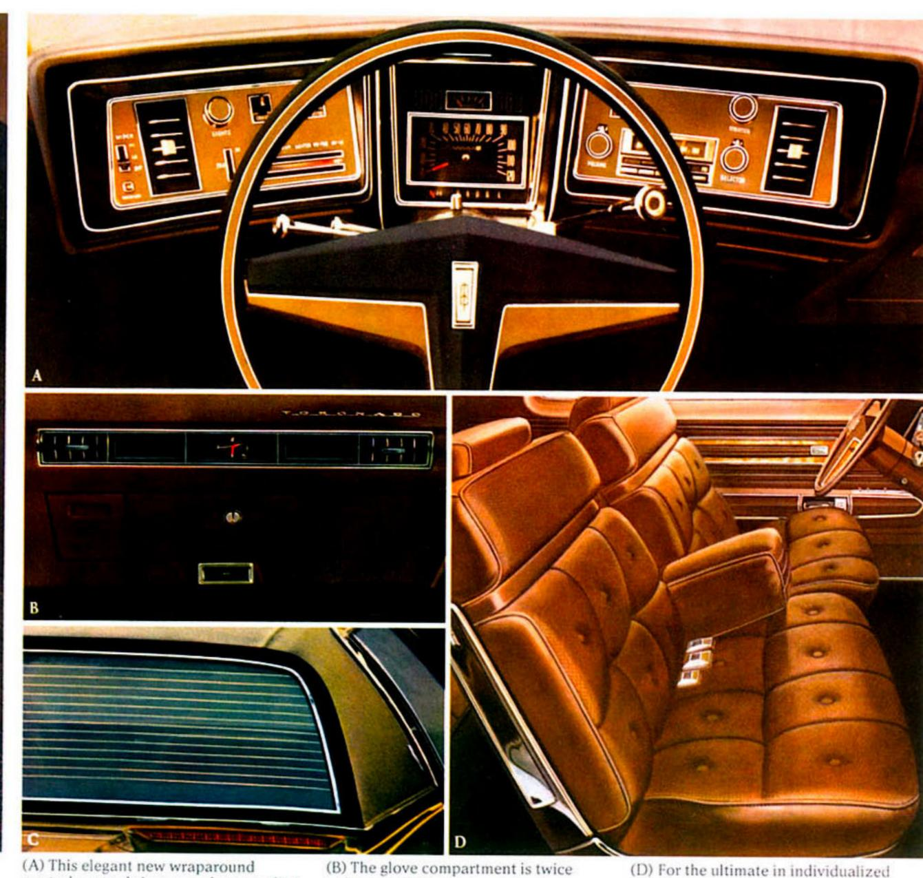
(A) This elegant new wraparound control center brings speedometer, fuel gauge and monitor lights together for quick and easy checking; and you can order a low-fuel warning light and trip odometer, if you wish.
