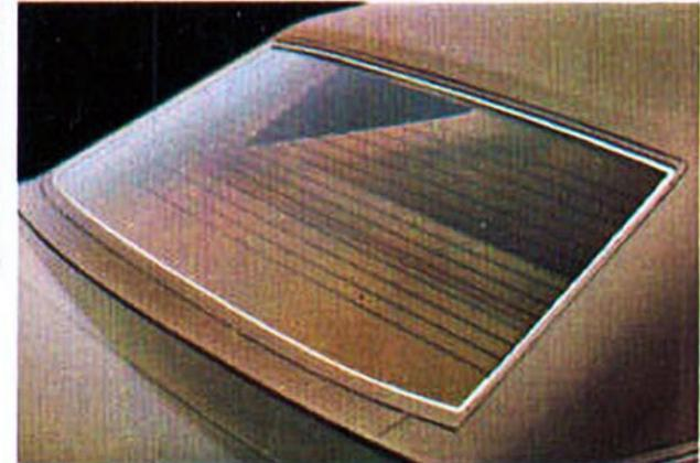
Rear Window Defogger. Very convenient. Remove fog and frost without leaving the driver's seat. Tiny electric filaments in the glass do the job silently. Available on most models. Blower-type available on Omega.
