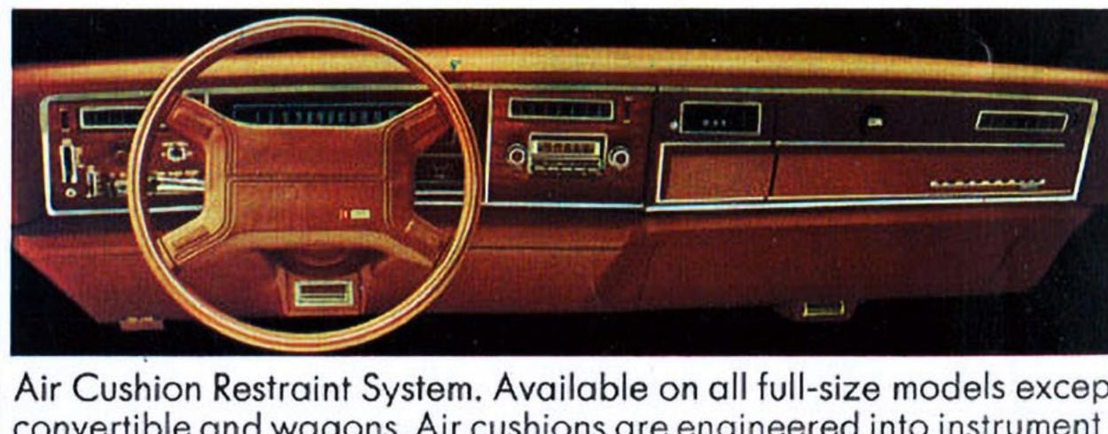
Air Cushion Restraint System. Available on all full-size models except convertible and wagons. Air cushions are engineered into instrument panel and steering wheel. When ordered, shoulder belts and starter interlock are eliminated from the seat/shoulder belt system.
