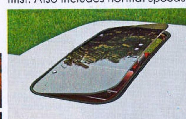
Vista Vent. Available on Cutlass Coupes and Supreme Cruiser. A window in the roof that helps ventilate when open. Lets in light, opened or closed. Features nonglare glass.
