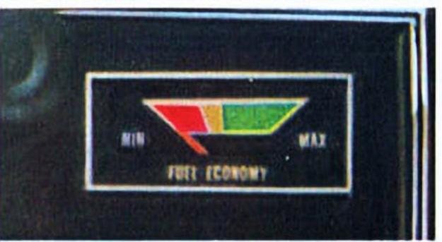
New Fuel Economy Gauge. This dash-mounted gauge shows you when you're attaining efficient gas mileage—and when you're not. Helps improve your driving habits, while improving gas mileage. Available on most models.
