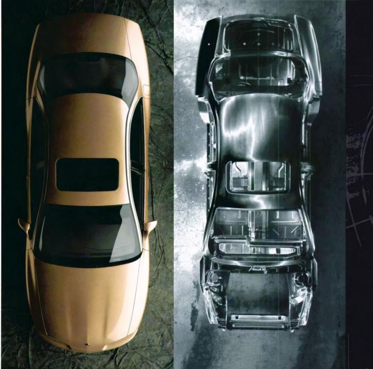
At the core of any true luxury performance sedan is a body structure of exceptionally high natural frequency, a measure of body strength. The stronger the body, the more solid the ride, the tighter the handling characteristics and the quieter the interior. Aurora engineers recognized this basic design goal as their first challenge. The result: Aurora's body structure is so strong, no car in its class surpasses the Aurora body structure's high natural frequency.
