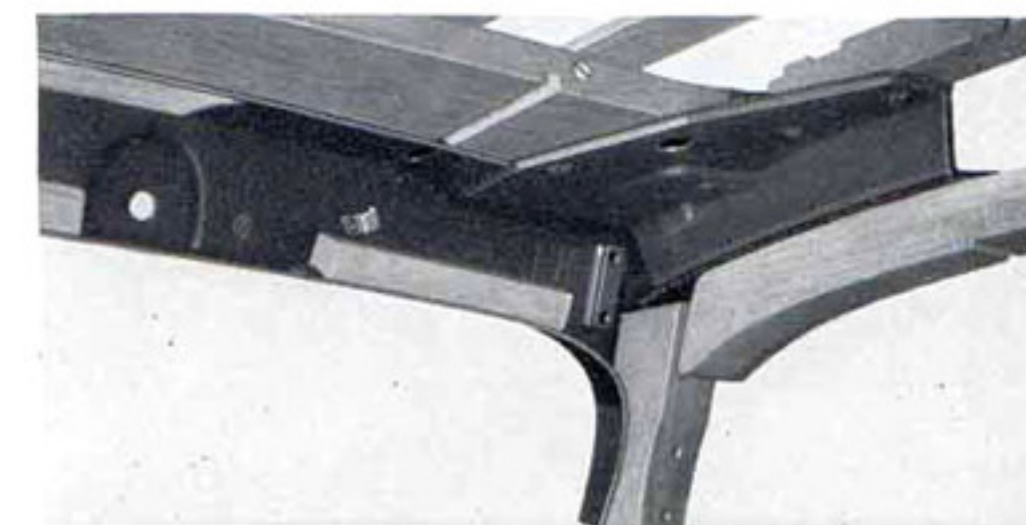
This heavy bracing between the front pillar and the top cross bar of the body frame is typical of the extra strength in all parts of Oldsmobile's Fisher bodies.
