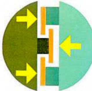
Self-Adjusting Brakes are now standard on all 1963 Oldsmobiles. They automatically reset themselves to proper clearance in the normal course of driving, make special adjustments unnecessary. New Durex sintered-metal wheel cylinders resist corrosion.
