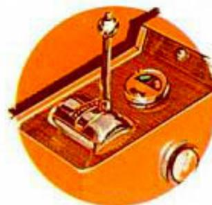
Turbo-Hocket Gauge on sport console shows performance range of the JETFIRE's engine.
