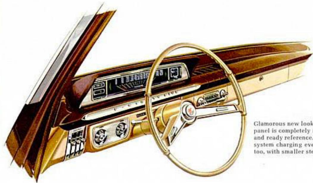
Glamorous new look behind the wheel! The F-85 instrument panel is completely restyled, places all gauges for quick and ready reference. New Delcotron generator keeps electrical system charging even at idle. Entry and exit is easier, too, with smaller steering wheel for increased clearance.
